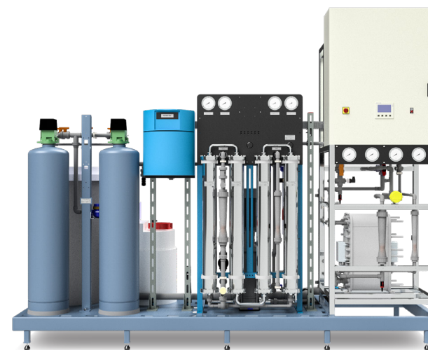
Figure 6 Frame mounted water treatment system for production of water suitable for electrolysis (<0.1 µS/cm). This system has a capacity of 1-2 m 3 /h equal to an electrolyser capacity of 5-10 MW.
